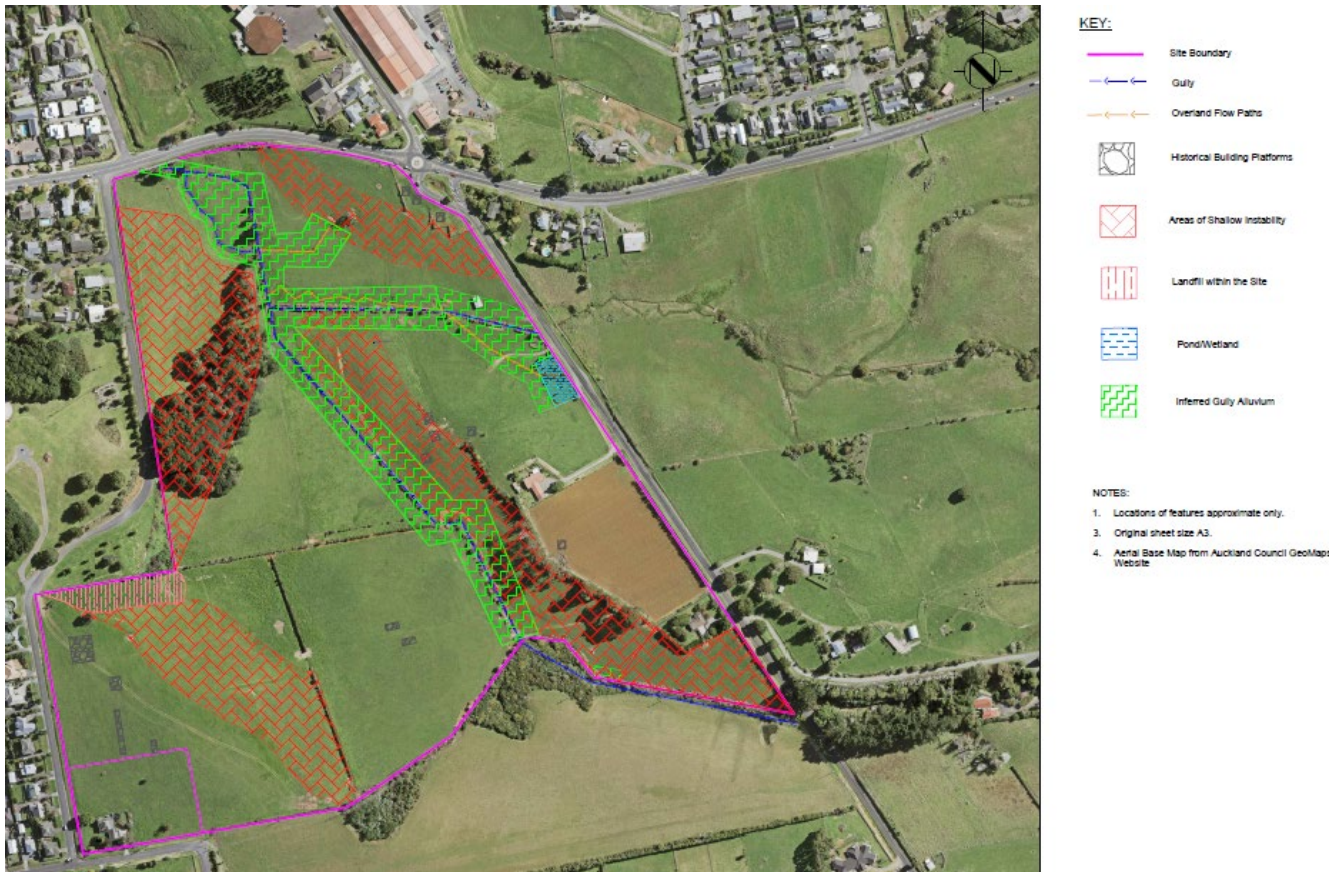
Figure 5 – Plan indicating the areas of instability across the Site. Source: Soil&Rock Consultants
